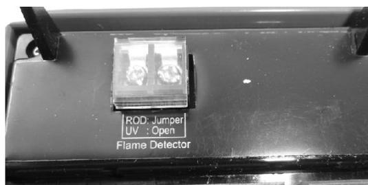
Fig. 4-4: Position of flame sensor selection jumpers on the back of the DBC1500.
