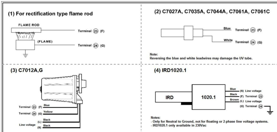
Fig. 4-1: Wiring a flame detector
