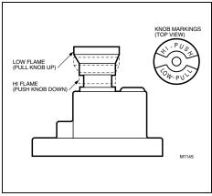
Fig. 10-HI and LOW settings for VS820D.
