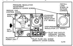
Fig. 3—Top view of standard capacity models.
