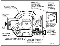
Fig. 4—Top view of high capacity models.
