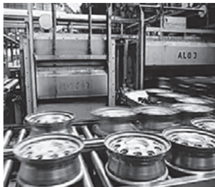
Aluminium industry: curing oven for wheel rims
