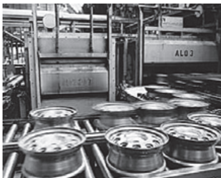
Aluminium age-hardening furnace with air/gas ratio controls for air deficiency cut-out
