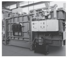
Shaft melting and holding furnace
