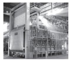
Bogie hearth forging furnace
