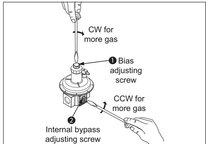
**Figure 4.10. Ratio Regulator with Internal Bypass Adjusting Screw**
