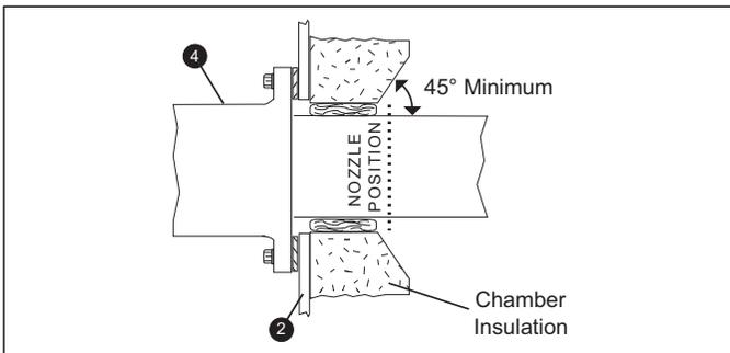
**Figure 3.3. Chamber Wall**
