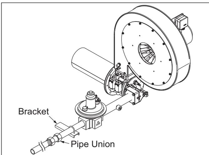
**Figure 3.9. Piping Connections**
