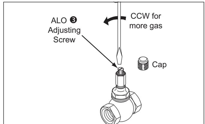
**Figure 4.12. Adjusting Limiting Orifice (ALO)**
