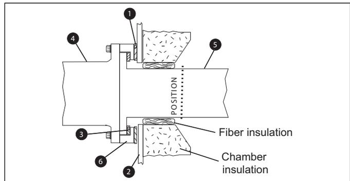
**Figure 3.5. Silicon Carbide (SiC) Combustor**
