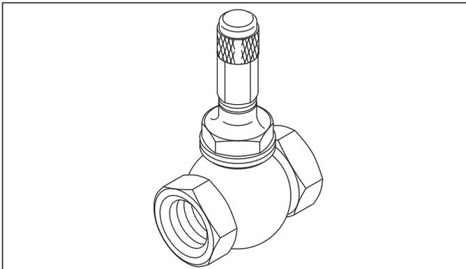
Figure 4.14. Adjusting Limiting Orifice (ALO)
