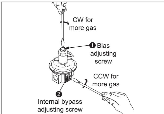
**Figure 4.16. Ratio Regulator with Internal Bypass Adjusting Screw**
