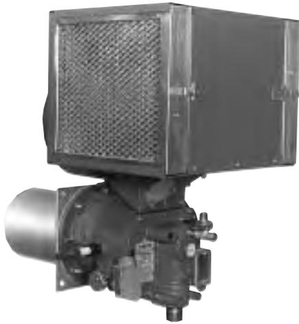
**Air filter assemblies** help to trap airborne particulate matter. They are offered with washable replaceable filter elements or with permanent metallic elements (as shown in photograph above). Filters mount onto OVENPAK® Burner's blower housing (or silencer housing of burners so equipped) and surround the blower motor and combustion air inlet.
