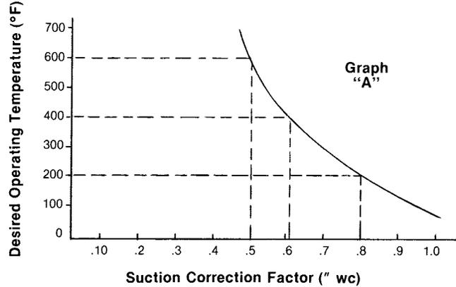
For example, if you anticipate running the system at 600°F, follow that dotted line to the right until it intersects curve, then read downward to a correction factor of 0.5. Therefore, if you read a cold suction of 1" wc, your expected suction "at temperature" would be 1" x 0.5 = 0.5" wc.
