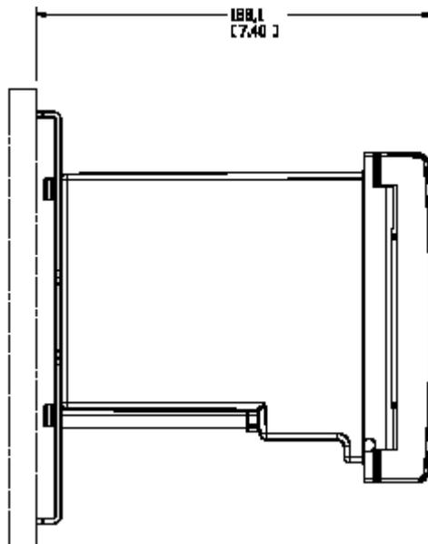
Figure 4 – Wall/Pipe Mounting Dimensions
