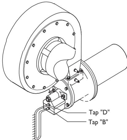
1. If the burner has and is ignited, set the main gas pressure regulator for 7" w.c. outlet pressure.
