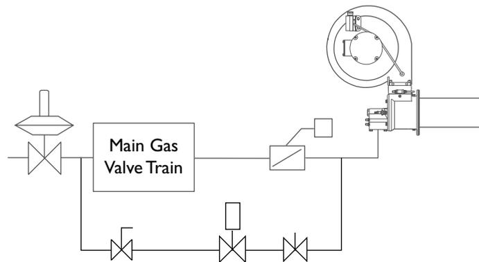
1. Drive the gas control valve to low fire.
